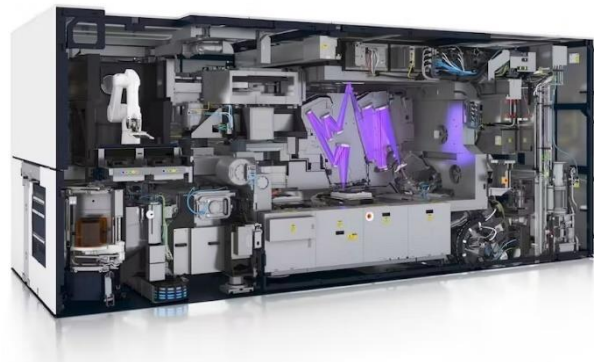
Figure (13) An ASML EUV lithography machine is shown. This is a complex machine with thousands of individual components originating from over 800 suppliers
