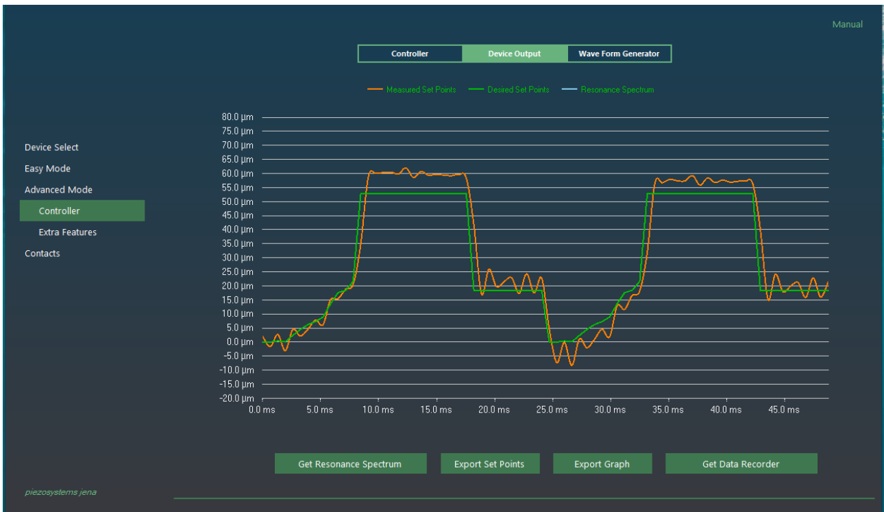
Figure 13 Amplifier feedback of the arbitrary waveform movement
