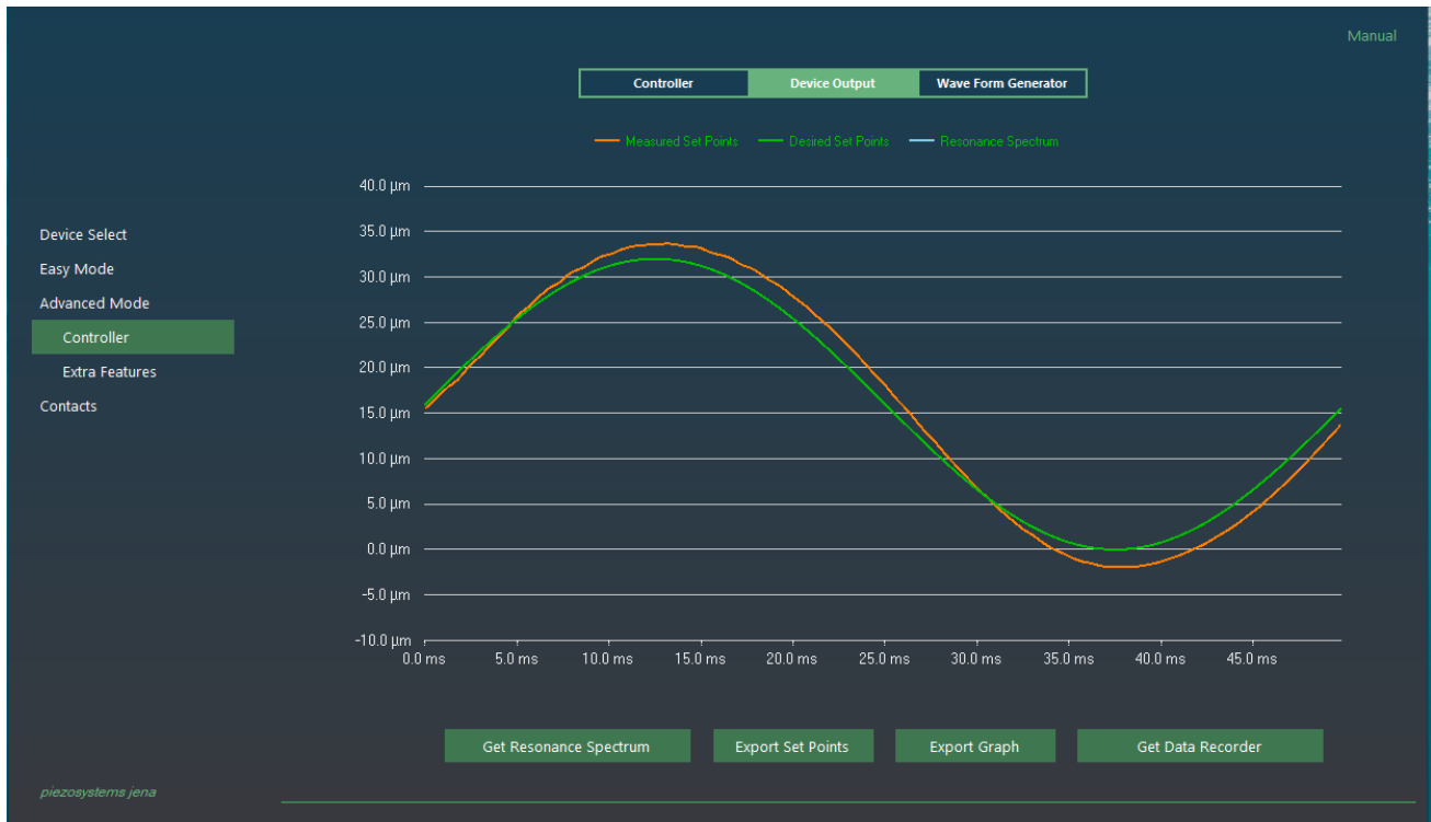
Figure 11 Wave Form generated movement feedback from the NV200D/NET
