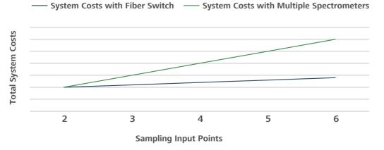
Using a fiber switch in-place of 3+ spectrometers will reduce your startup costs from day 1.
