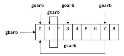
After the command grun,1 the arbitrary waveform generator starts at the index defined by goarb and runs until the index defined by gearb. In all successive cycles, the arbitrary waveform generator starts at gsarb. This is repeated until the number of cycles reaches the value given by gcarb.
