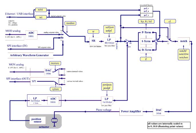
The PID-controller can work in two different modes: The open loop mode (OL) and the closed loop mode (CL). The setpoint can always be given by USB, Ethernet, arbitrary waveform generator or analog input. The slew rate, low pass and notch filters can always be used to avoid excitation of system resonances or to limit the setpoint dynamics in order to provide a trackable motion profile to the power amplifier and the actuator.
