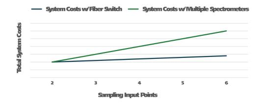
Using a fiber switch in place of 3+ spectrometers will reduce your start-up costs from day 1.
