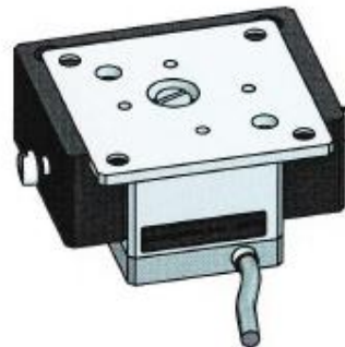
Fig: Using of the mounting tool (part. no. K-190-00) with top plate type "B" (size: 38x38mm 2 )
