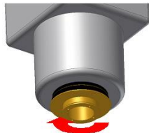
2. Screw the Flex-Adapter into the microscope
