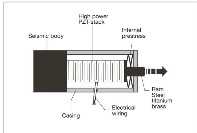
**Figure 6a:** Schematic of a single output piezo-shock-generator.
